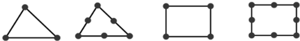
3-node Triangular 6-node Triangular 4-node Quadrilateral 8-node Quadrilateral
