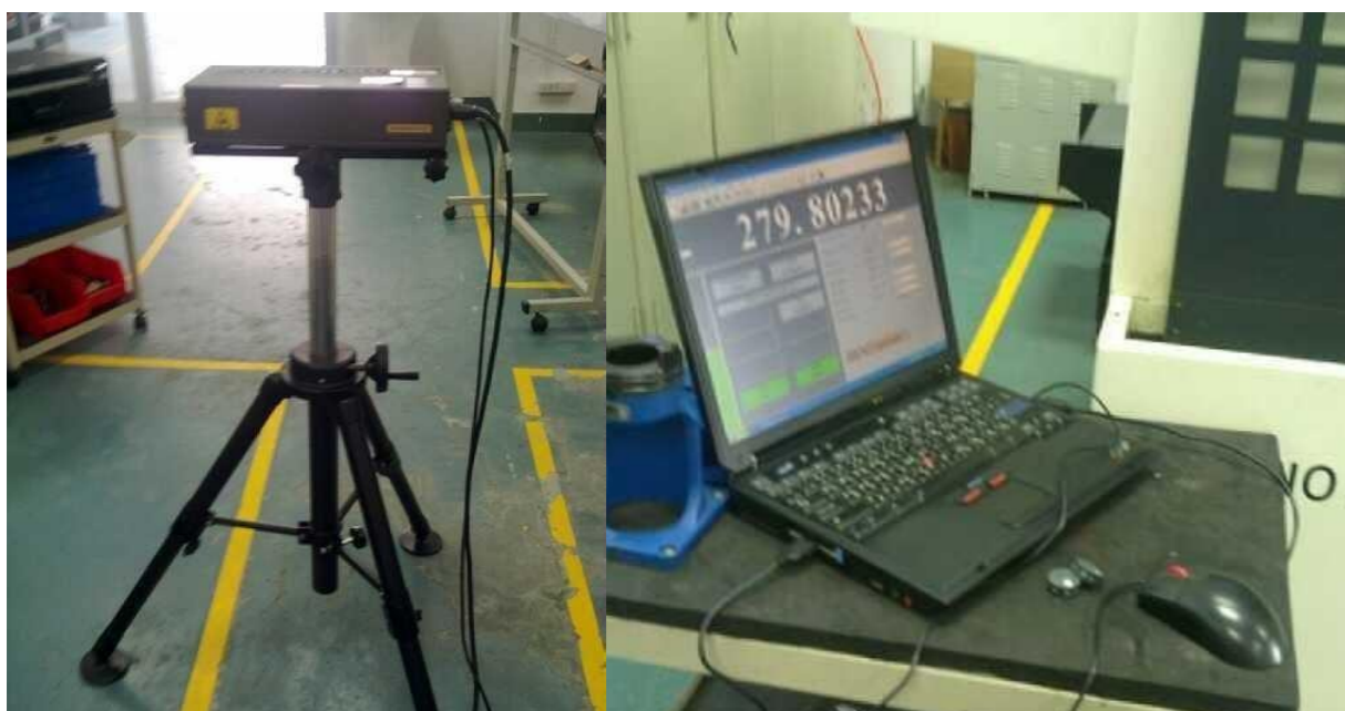
Machine Precision with Laser Interferometer
